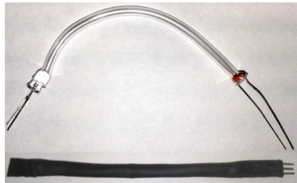
Fig. 3. Stages of manufacturing an optical bending sensor
