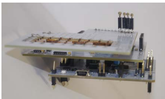
Figure 19: Nucleo F411RE, Drive and Core Shield (Front View)
