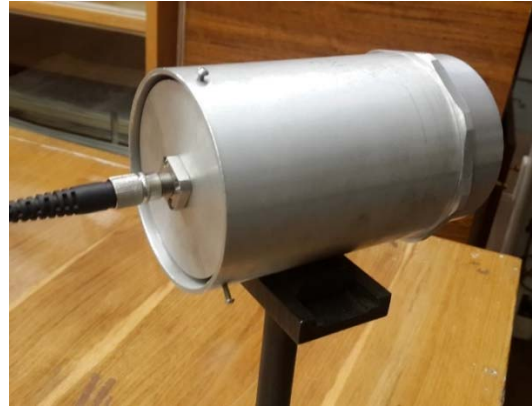
Figure. 3 – System for fixing the end of a fiber with a threaded tip of the "FC" type
