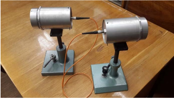
Figure. 2 – Fiber-optic transmission system for analyzing signals
