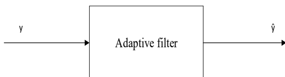
Figure 1- Schematic representation of the filter where: y – the measured value, \hat{y} – estimate the required values
