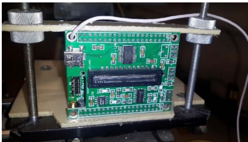
Figure. 7 – spectroscopic information reading device
