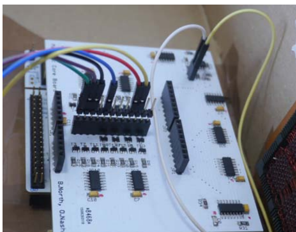
Figure 26: Connections for addresses 4 and 14 on the Drive Shield
